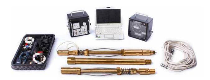
This system was built to control HDD process with big depth and length. Working principle is based on measuring of gravity and magnetic field of the Earth using special sensors in the probe. All data goes by cable to the Interface module of the system for decoding. From module data goes to PC where it is calculating to define depth, probe position, angle etc. Final information is assembling to convinient table and goes to Control Panel of Drillmaster.
